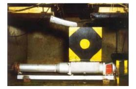
A custom-built W082 is speeding up waste disposal at a Scottish tannery. Previously the 'fleshings' were shovelled manually from the processing area to a skip, this method was highly labour intensive. The cast iron W range pump with large auger and hopper were specially modified in order to handle this difficult material. The fleshings waste is gravity fed into the hopper, then pumped at 5.5m3/h at a pressure of 3 bar, along 30m of pipe direct to an outside skip for disposal.
