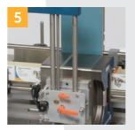
Hot-foil or thermal transfer printers can be easily integrated in order to print variable data.
