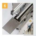
The 152C masters various mounting conditions and production environments. The conveyor belt is available with a width of 100 or 150 mm, at a length of 1,540 mm.
