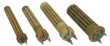
Replaceability constitutes an essential difference to all other heating elements used. Gräff ceramic sectional heaters are positioned in protective pipes made of stainless steel or steel; these protective pipes can be welded in, screwed in or flanged on a container. The heating elements can be replaced at any time without having to drain the medium from the container.
