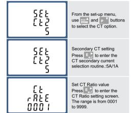
For example, if using a 100/5A current transformer you
