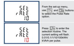
Use MD/A and P buttons to choose pulse rate. On completion of the entry procedure, press
