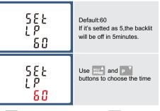
Press [] to confirm the setting and press [] to return to the main set up menu.
