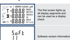
The first screen lights up all display segments and can be used as a display
