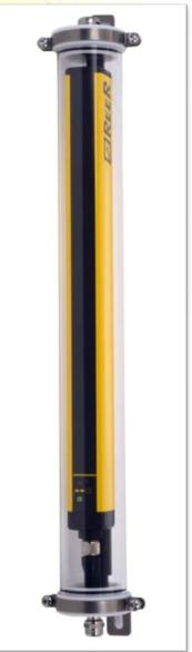
The small EOS WTF and WTHF cylindrical enclosure (only 56mm diameter) is IP 69K protection rate tested and can withstand up to 80 bar of water jets pressure at the temperature of 80°C.
