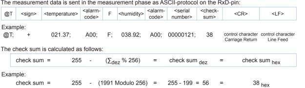
The check sum is not transmitted as a hexadecimal character with 1 byte, but is translated into readable digits with 2 bytes. Through the comparison of the transmitted check sum with a check sum calculated at the read-out point, the user has the opportunity to check whether the transmission of the data is error-free.
