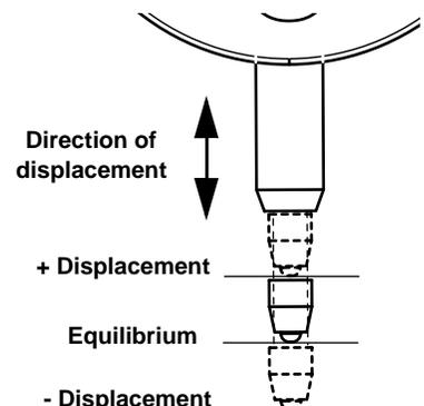
If the object will be displaced both positively and negatively from its equilibrium position, adjust the indicator so that the position of the measurement head when it is in contact with the object is about halfway between the limits of the measurement head's travel. Press and release the ON/O button to zero the indicator when the measurement head is at the equilibrium position.
