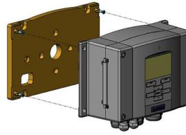
Mounting with DIN Rail Installation Kit
