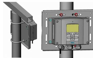
Mounting Rain Shield with Installation Kit
