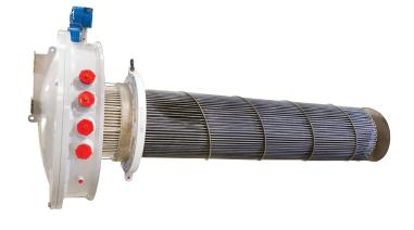
The HELIMAX™ is a next generation heat exchanger with Continuous Helical Flow Technology™ that enables ultra-high heat transfer unlike large, traditional heat exchangers with dead zones. Fluctuations within the heat exchanger to either the sheath temperature or the localized flow rate are common causes of coking, which can lead to system failures and expensive downtime.
