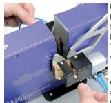
Using a special fixture to manually rotate the part, the diameter can be measured over 360° of the circumference to precisely measure the maximum MAX-D, the minimumMIN-D and ovality which is really MAX-D - MIN-D.
