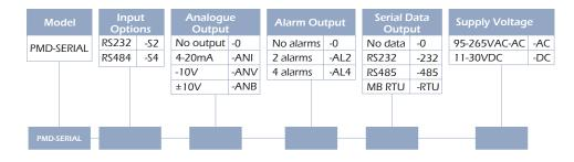
Example - PMD-SERIAL display with RS232 input, 4-20mA output, 2 alarms, RS485 output and 110V AC powered. **Order code will be: PMD-SERIAL-S2-ANI-AL2-485-AC**
