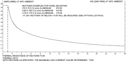
IS THE MAXIMUM LOAD CURRENT POSSIBLE WITHOUT EXCEEDING THE DEVICE RATINGS
