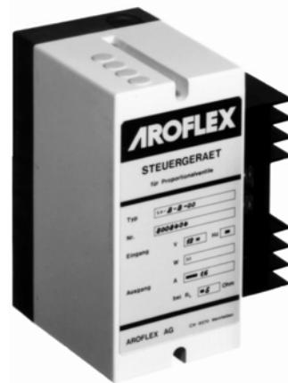
The current stabilising control box SA controls the DC-solenoids of analogue valves (proportional valves) supplying a constant current, independent of coil temperature and resistance.
