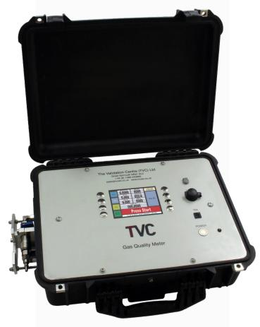
The GQM features a 5.7-inch LCD screen for a clear view of the measured parameters. It is a simple and easy-to-use system which can be configured to measure Oxygen, Helium, Nitrogen, Carbon Dioxide, moisture, and can calculate Argon levels. The gas level data is logged directly on to a 4GB pen stick flash drive along with the test date and time.
