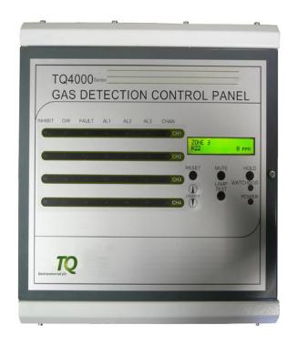
The **TQ4000** unit is a 1-4 channel control unit for use in conjunction with toxic, flammable, Oxygen and other 4-20mA gas sensors. The unit has been designed and manufactured in the UK to offer A low cost, highly reliable solution to gas monitoring. The unit can be factory or field configured for 1 - 4 channels as toxic or flammable sensors or a combination of gas and other 4-20 mA sensors.
