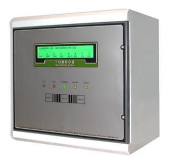
The standard **TQ8000** is an 8 channel stand-alone control unit, which can be expanded up to 48 channels for larger installations. Capable of monitoring inputs from a wide variety of Gas Detectors and many other 4-20mA output devices, such as temperature and pressure.
