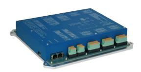
boards. The main board provides high CPU power, large DRAM and FLASH memory as well as modern communication interfaces. The I/O boards are small in size and are configurable by software. They can be attached in different number and type to the main board.
