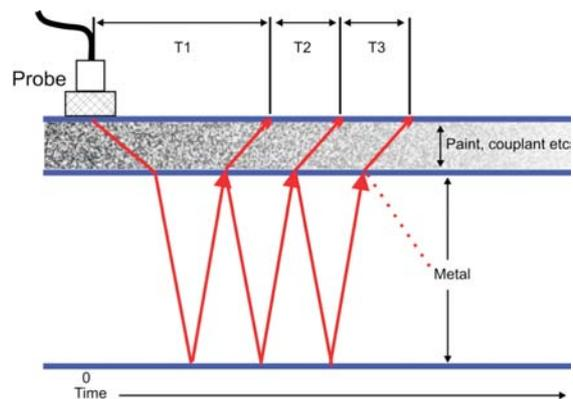
With multiple echo, readings are taken by measuring the time delay between any three consecutive backwall echos. The time of T1 (coating thickness) is ignored. The times of T2 and T3 are equal to the time that it takes to travel through the metal. Only by looking at three echos can the measurements be automatically verified (where  $T2 = T3$ ).
