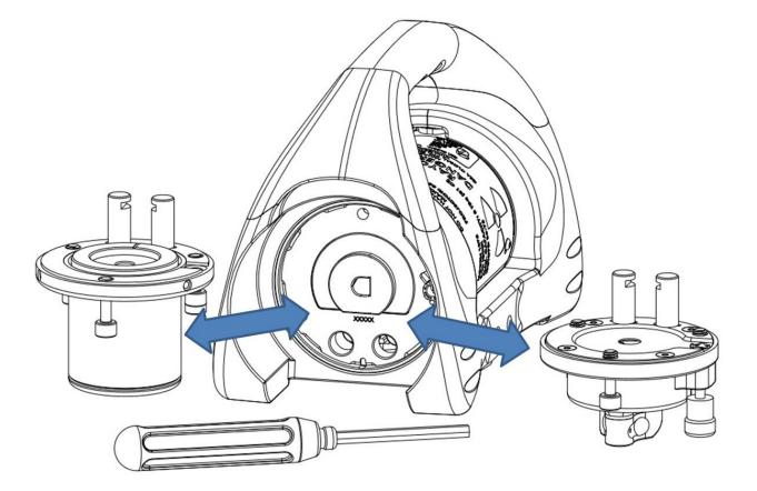
Figure 5 – SENTINEL 1075 SCAR Pro with Outlet Port Assemblies Removed
