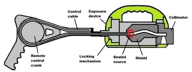
Figure 11 – SENTINEL 1075 SCAR Pro in SCAR Mode – Source Secured
