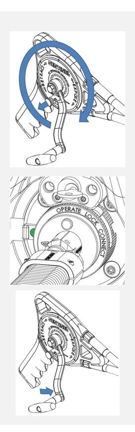
**NOTE:** Any residual force on the control cable from the crank when the source is locked could cause the source to move slightly after unlocking the lock slide for the next exposure.
