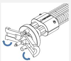
**4.** The protective cover will disengage from the exposure device.
