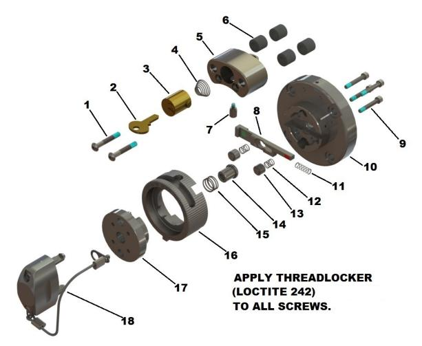
Figure 17 – Collimator Assembly Component Exploded View
