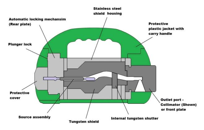
Figure 3 – SENTINEL 1075 SCAR Pro Gamma-Ray Source Projector
