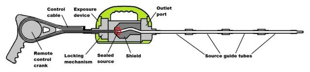
Figure 7 – SENTINEL 1075 SCAR Pro in Projector Mode (Source Secured)
