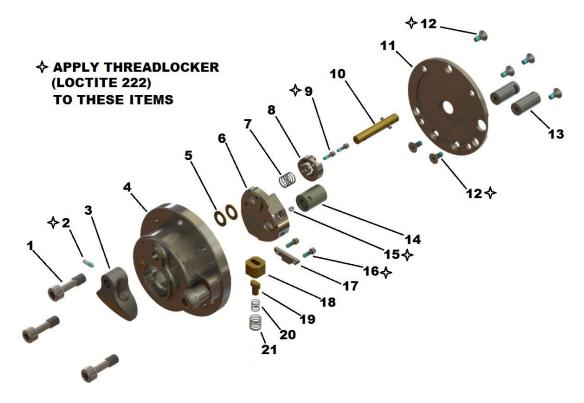
Figure 15 – Front Plate Assembly Component Exploded View
