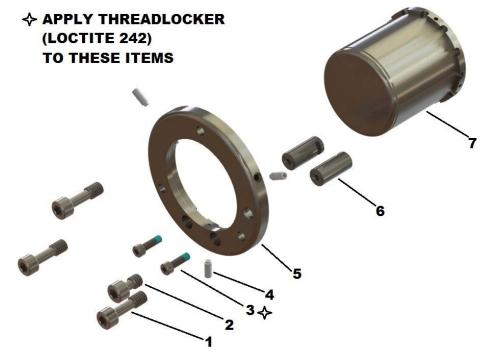
Figure 16 – Collimator Assembly Component Exploded View
