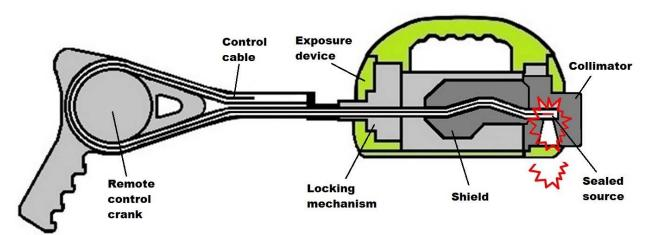
Figure 12 – SENTINEL 1075 SCARPro in SCAR Mode – Source Exposed
