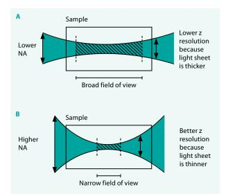
**Figure 2:** By adjusting the shape of the light sheets, illumination is tailored to sample size and imaging goals. A lower NA results in a broad field of view (A), and a higher NA results in a narrow field of view (B). While there is a tradeoff between the field of view, the thickness of the light sheet, and the z-resolution, the UltraMicroscope II allows balancing these parameters to meet your specific requirements.
