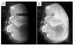
**Figure 1:** Unidirectional illumination (from the left) results in dark areas and stripes as parts of the sample are not exposed to the light sheet (A). The bidirectional, triple light sheet illumination of the UltraMicroscope II generates a clear, evenly illuminated image (B).
