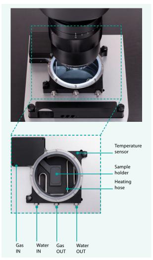
Figure 4: The *in vivo* sample chamber maintains constant temperature and  $CO_2/O_2$  concentrations for functional and time-course imaging.
