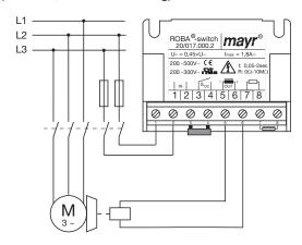
AC-side switching means **low-noise switching**; however, the brake engagement time is longer (approx. 6-10 times longer than with DC-side switching), use for non-critical braking times.
