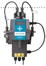
WTW's Turb PLUS 2000 continuously monitors turbidity in drinking water using DIN EN ISO 7027 or EPA 180.1 compliant method. Equipped with ultrasonic cleaning.
