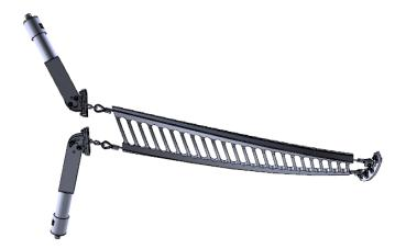
The <u>CleanScrape® Cleaner</u> is mounted diagonally on the discharge pulley and forms a three-dimensional curve. The cleaner has a matrix of carbide scrapers incorporated into the main rubber body during the vulcanization process. Despite a relatively low contact pressure between the belt and cleaner 85 to 95% of the adhering material is removed.
