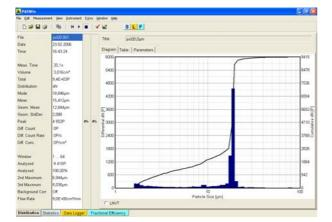
Main Window of the Particle Analyzer Software PASWin showing a high-resolution size distribution diagram of monodisperse particle material Based on calculation methods and calibration functions from channel content histograms of particle counters, particle size distributions can be calculated. Data are presented as graphics, tables or on screen or printer and stored as ASCII files.
