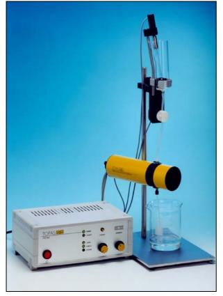
Particle Analysis System for Fluids FAS 362
