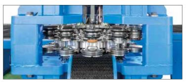
12 Tool stations with cassettes for automatic tool change with easy exchangeable cassettes for punch, stripper and die.
