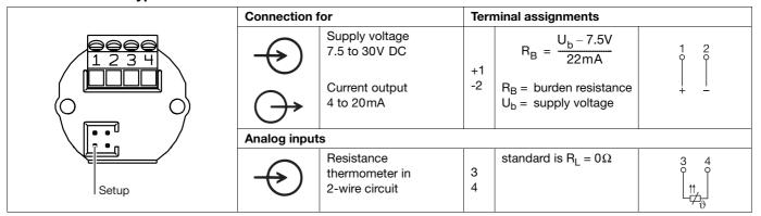
Caution: the maximum torque of the screw terminals is 0.15 Nm.
