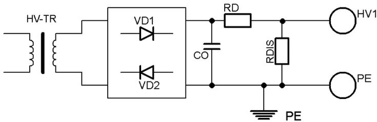
Figure 1: Electrical wiring of the high voltage output, device class GPS 350W - COMPACT
