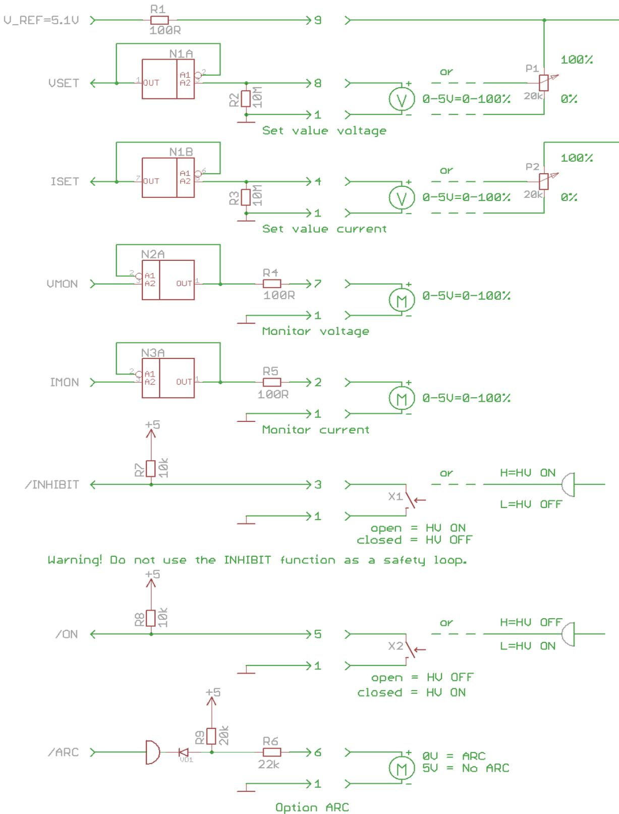
Figure 15: Wiring of analog and digital inputs and outputs
