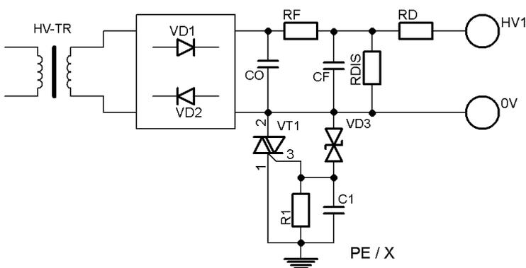
Figure 2: Electrical wiring of the high voltage output, device class GPS 300W and 800W
