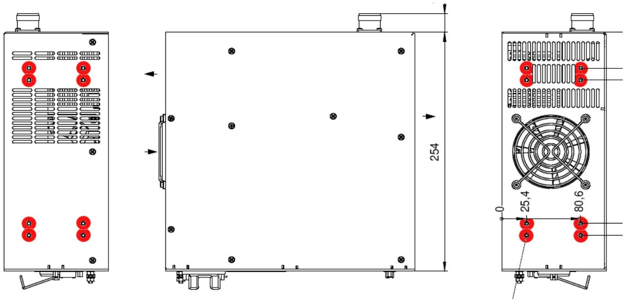
Figure 7: Mounting points on both sides e.g.  $V_{nom} > 40kV$
