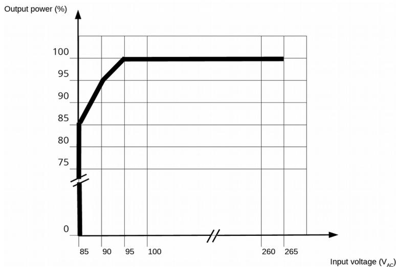
Figure 13: Power reduction vs. input voltage
