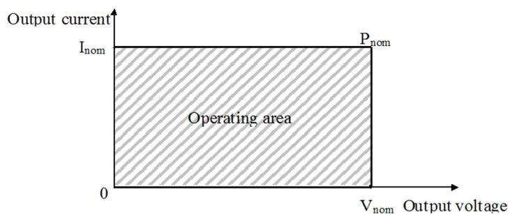
Figure 12: Operating area of the device
