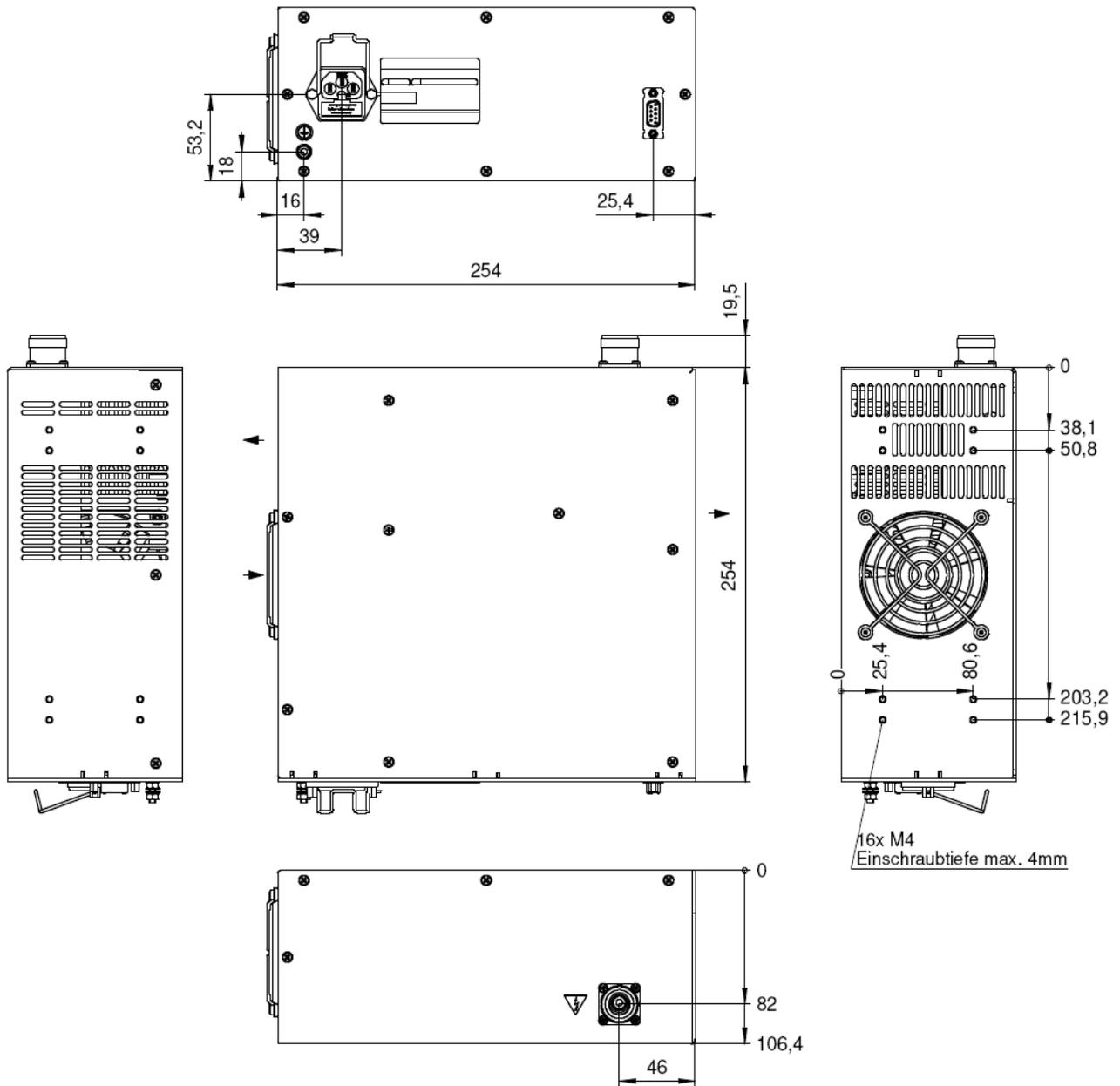
Figure 6: GPS 350W – COMPACT 40 kV  $\leq V_{nom} \leq 70$  kV
