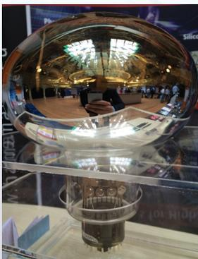
iseg PHQ modules are developed as direct HV supply of modern photo multiplier tubes (PMT) with the high voltage power supply integrated in the PMT socket.
