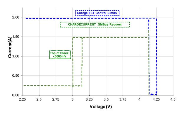
NOTE: The charging current requested from 3.0 to 4.2 V is defined by the temperature of the pack as shown in the preceding charge operating limits graph in this section. A 1.5A charge current is shown in this graph to represent the current defined by said graph.
