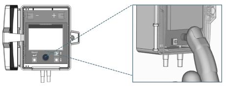
There is a capacitive button under the cover (see picture). With an immediate touch on the cover the display can be turned on without the cover must be opened. The display remains on for 10 seconds (not adjustable).
