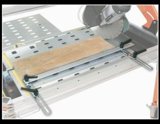
**SIDE BAR SUPPORT** Made to have the top precision during the execution of straight and angled cuts on slabs of large size. Adjustable angle-shot cut.
