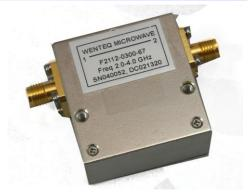
F2112-0300-67 is a single junction coaxial isolator with SMA female coaxial connectors operating in the frequency range from 2.0GHz to 4.0GHz and offers 0.6dB maximum insertion loss and 18dB minimum reverse isolation at room temperature. The coaxial isolator can handle 30 watts of forward CW power and 10 watts of reverse power.
