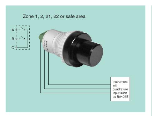
The BA490 encoder is a robust panel mounting rotary control knob with a quadrature switch contact output, suitable for installation in hazardous or safe process areas. It is designed for easy adjustment by a gloved hand and may be directly connected to almost any instrument that accepts a three-wire quadrature input to provide a simple way of making adjustments from within the process area.
