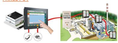
RS485 Bus / 1 km / fitted with 64 modules as a maximum
