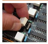
The LEDs are fitted on detachable sockets, enabling a change of colour. The colours available are the following ones:
