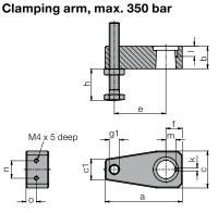
Clamping arm complete with angle
