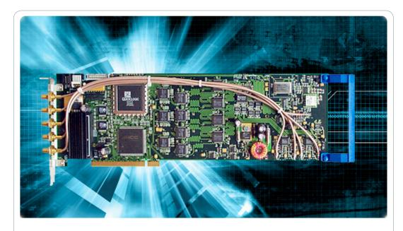
The Model P7888 Series are one of the fastest commercially available multiple-event time digitizers with up-to four inputs. They can be used as an ultra fast Multiscaler/TOF system in Time-of-Flight massspectrometry and time-resolved single ion- or photon counting.
