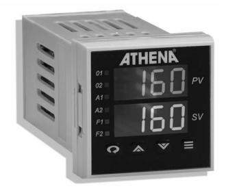
The Athena Legacy 16 is a 1/16 DIN panel mounted, auto-tuning controller that can be used for precise control of a single loop with two independent outputs. The controller accepts thermocouple, RTD, voltage, or current input. RS-232 or RS-485 communications are available, and two digital LED displays provide visual indication of various controller functions.
