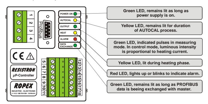
In addition to the functions shown in the diagram above, various controller operating states are indicated
