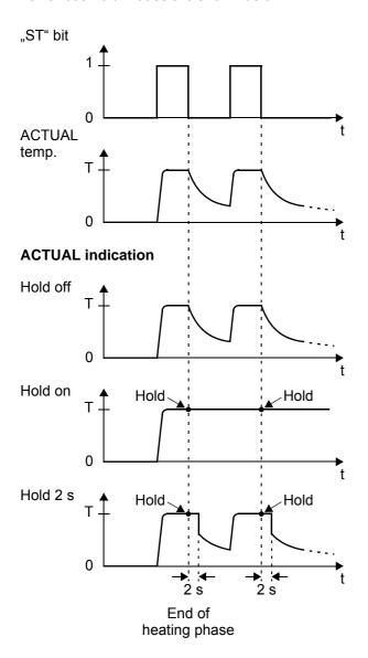
The "Holde mode" function must be activated by means of the PROFIBUS parameter data (\$ section 10.7 "Parameter data" on page 30) or the DPV1 protocol extension (\$ section 10.8 "DPV1 protocol extension (as of GSD Version v2.0)" on page 35). (default setting: Hold mode off).
