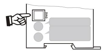
Only a ROPEX comunication interface is allowed to be connected to the diagnostic interface. Connecting another device (e.g. a telephone cable) could result in malfunctions or damage to the controller.
