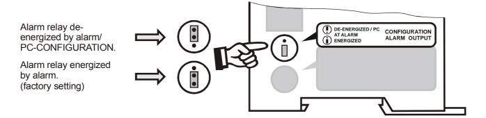
If the jumper is not inserted, the alarm relay is permanently energized when using a controller up to production date January 2006. The other functions of the controller (e.g. heating, AUTOCAL etc.) are not impaired by this.
