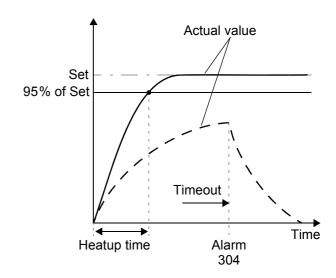
The "Heatup timeout" function must be activated by means of the PROFIBUS parameter data (\$\scale=\text{ section 10.7 "Parameter data"} on page 30) or the DPV1 protocol extension (\$\scale=\text{ section 10.8 "DPV1 protocol extension (as of GSD Version v2.0)" on page 35).
