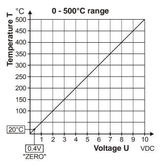
An indicating instrument can be connected to this output in order to visualize the temperature of the heatsealing band.
