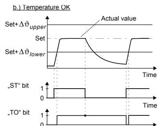
For controllers with software revision 100, 101 and 102 the configuration for the "TO" bit can be set via the ROPEX visualization software. As of software revision 103 the configuration for the "TO" bit is set in the PROFIBUS parameter data (or the DPV1 protocoll extension). A configuration with the ROPEX visualization software is no more possible.
