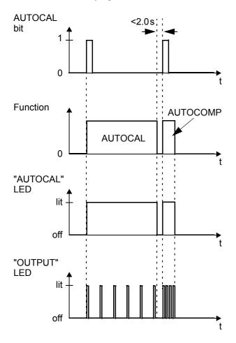
The "OUTPUT" LED blinks repeatedly when the "AUTOCOMP" function is executed and the actual value output (terminals 17+14) is set to 0...3°C (i.e. app. 0 VDC).
