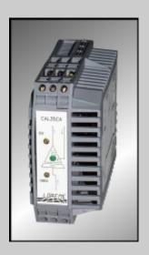
The CAL35CA measurement converter allows to transform alternative voltages or currents into a current (0 ... 4 ... 20 mA) or a voltage (0.....10 V) proportional to the input value.
