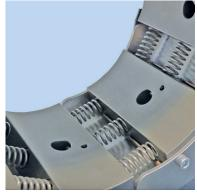
Due to our long master dies, you can crimp virtually all types of fittings. This slide bearing technology reduces friction by 20% and ensures high process stability and reproducibility.
