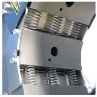
Due to our long master die, you can crimp virtually all types of fittings. This slide bearing technology reduces friction by 20% and ensures high process stability and reproducibility.
