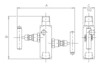
The 'G12' Type 2 valve manifold is designed for remote mounting to static pressure transmitters. The separate vent valve gives full control of venting of the instrument, plus the ability to calibrate in-situ. Each needle valve head is designed for safe and reliable isolation, giving bubble tight shut off, with non-rotating & anti-galling tip and dynamic self-adjusting spindle seal to give long service life in a variety of service conditions.
