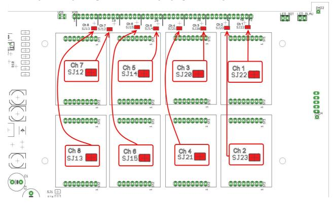
For closed solder bridges, connecting quarter bridges to 350 ohm is possible. The use of half and full bridges is also possible with closed solder bridges. The measurement result for full bridges is then displayed too small by approx. 1% to 2%. Optionally, the measuring amplifier is supplied with 120 ohm or 1000 ohm bridge completion.
