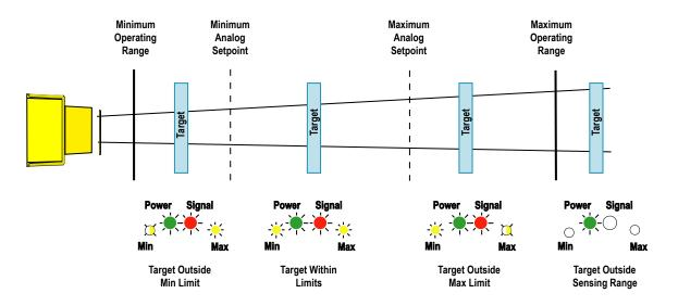
Figure 5. Status Indicator Conditions for Each Target Position
