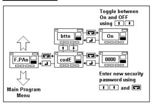
The front panel controls referred to here allow the operator to set a security access password (or change an existing one) and to switch on the anti-tamper feature - "bttn". If "bttn" is set to "on", then the buttons are enabled, if set to "off" then the buttons are disabled (to re-enable see section 8.7).
