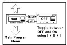
**8.5.2) "rESn" - Display Resolution**. This function selects the resolution of the least significant display digit. It may be set to 1,2,5 or 10. This function can be useful if the source signal is noisy. E.g. setting a display resolution to 5 would mean the display only increases or decreases in steps of 5 digits, thus "smoothing" the display.
