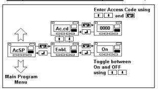
allows an operator access to the alarm setpoints without having to go through all the other programming menus. When this function has been enabled, pressing the scroll and up button together will give the operator access to the setpoints. This function can be password protected by setting an "Access Code" (Ac.cd). It is possible, if desired, to use the same password for access to both the alarm and main menu programming.
