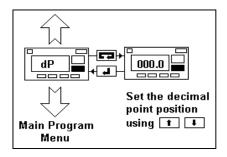
**8.5.4) "hLd"- Max and Min Hold.** Whether this parameter is set to "On" or "OFF", the maximum and minimum display is always being monitored and stored in the max/min register. In Normal Display Mode with the parameter set to "On", the maximum and minimum can be displayed (by pressing the up and down buttons) and reset (by pressing the up and down buttons together). The maximum and minimum values are lost if there is a power failure.
