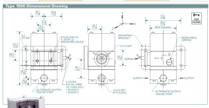
The Type 1000 has long been a standard in the I/P & E/P industry. With a built-in booster, the T-1000 provides a flow capacity up to 12 SCFM, making it a versatile transducer for many applications.
