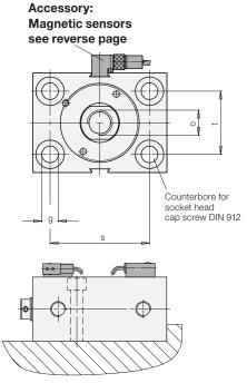
Cylinders must be backed up for operating pressures exceeding 160 bar.
