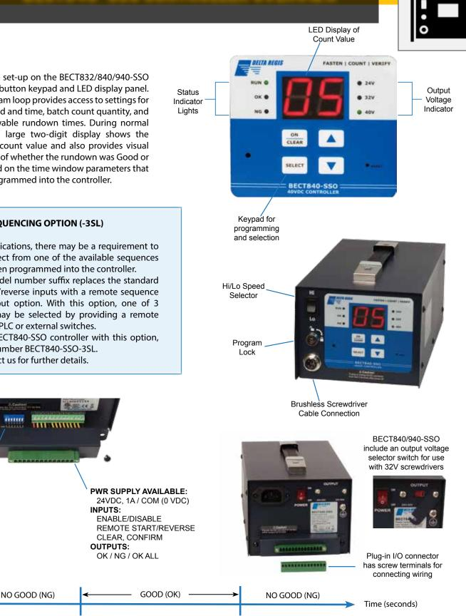
If the fastening cycle completes (clutch trips) within the programmed time window, the rundown cycle will be accepted as GOOD (OK) and the batch count will increment. A rundown outside the time parameters will result in a NG output.
