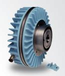
The driving part is linked to the unit through two ball bearings, it is provided with a cylindrical area with axial threaded bores for an easy coupling of a pinion or a pulley (see assembly examples **const. 1.1**) or of an elastic coupling to be adapted between two shafts in line (**const. 1.2**).
