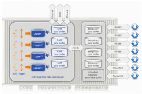
According to the configuration of up to 4 loggers occurs the logging of the buffer data at a selectable medium (intern. Flash, USB, SD-Card) with selectable logging rates, storage duration, start and stop trigger (auto start, condition, touch) with or without preand post-trigger.
