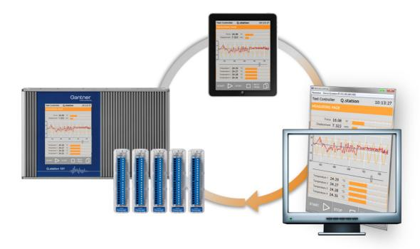
Due to the separation of real time and user tasks of the controller (real time kernel, user kernel) it is warranted that pretentious high speed tasks like dynamic logging or fast PID will run stable and independent from the very flexible and individual tasks like visualization and operation.
